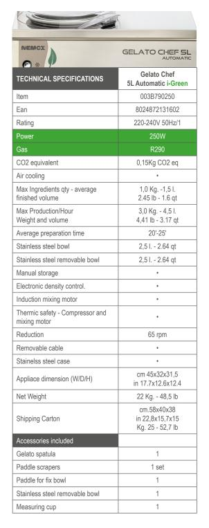
Simply activate the storage switch. The production cycle will star and, when the ice cream will be at the right consistency, the storage cycle will be activated. A dedicated software manages to start and stop the mixing paddle and compressor depending on the ingredients' density in order to keep the ideal consistency for serving.
