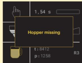
If the hopper is incorrectly positioned or missing, the dose cannot be delivered and the warning message «Hopper missing» appears on the screen.
